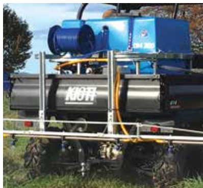
OPTIONAL SMART-FIT BOOMS, ALLOWING TAILGATE TO REMAIN CLOSED
