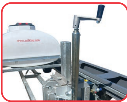
Front to back and sideways levelling system.
