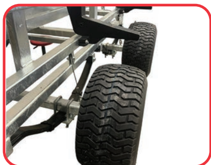
High load carrying in tandem axle design.
