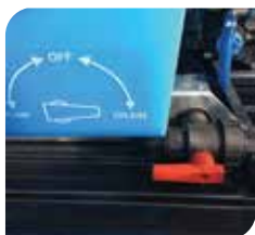
3-WAY DRAIN TAP: PUMP, OFF AND DRAIN
