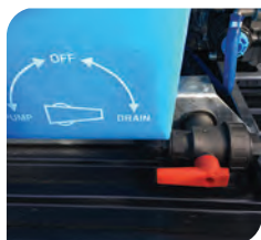
3-WAY DRAIN TAP: PUMP, OFF AND DRAIN
