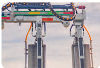
HYDRAULIC ROW ADJUSTMENT (2.4–3 Metres)
